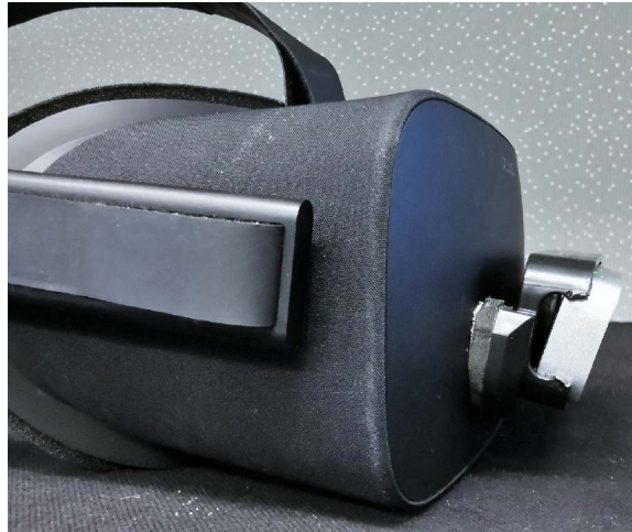
Figure 2.1: A Leap Motion Controller was attached to the front of the Oculus Rift at a 20^\circ down angle to increase its field of view when the user's head is upright.
