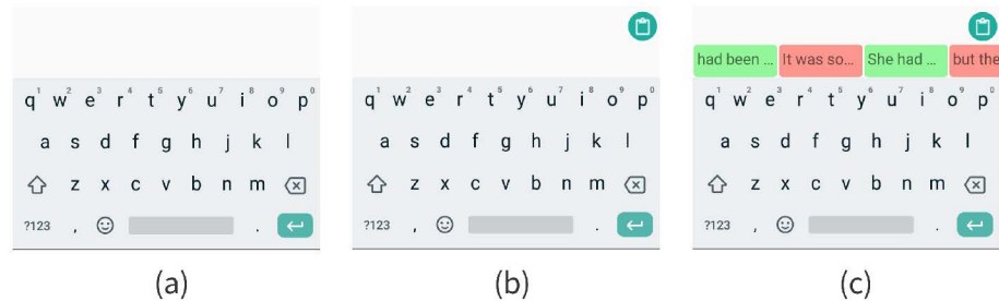
Figure 4.6: Different states of GeShort’s floating clipboard: (a) the clipboard icon is not visible when it is empty, (b) the clipboard icon appears when it has content, (c) tapping on the icon displays recently cut and copied text in a bar above the keyboard, highlighted in red and green backgrounds, respectively.
