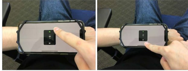
Figure 2.2: Input stepper is the default number picker on most smartwatches: it displays a full-screen number wheel that users spin by flicking up or down to increment or decrement a numeric value, respectively.
