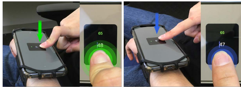
Figure 2.5: Force-based number picker: the user applies extra force to increment and soft force to decrement a numeric value.
