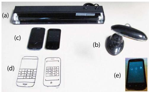
**Figure 15. Instruments used during the second study: (a) black light, (b) jumpstart LED lamp, (c) Samsung Galaxy S III and Symphony Xplorer W60, (d) transparent sheets with tracings for the above mentioned devices, and (e) in the inset illustrates how smudges often glow under black light.**
