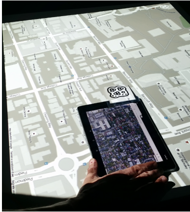
Figure 3. A sample application: the mobile device is tracked on an interactive surface exploiting the reactIVision fiducial markers [8]. The mobile device displays an additional layer of information for the digital map rendered on the tabletop. For tracking the position of the tablet, we exploit the capability of the tabletop device to recognize reactIVision fiducial markers and use the TUIO protocol [8] to transport all the relevant information, such as the position, speed, and rotation.
