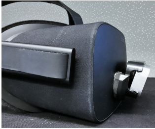
Figure 1: A Leap Motion Controller was attached to the front of the Oculus Rift at a 20° down angle to increase its field of view when the user’s head is upright.
