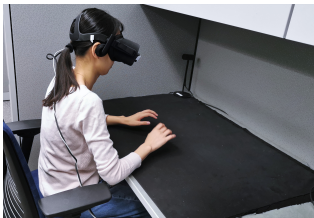
Figure 2: The setup used in the study. The black material on the desk is duvetyne 4 .
