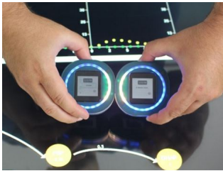
Figure 4: Two Actibles in an off-table interaction in the Active Pathways application. Each Actible is bound to a molecule and touching them together creates a reaction between the two molecules.
