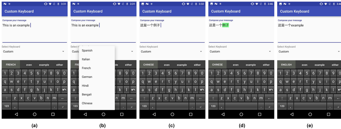
Fig. 1. The proposed real-time translation method: (a) the user types as she usually would. Her default translation language is French, thus tapping on the language button will translate the input to French, (b) but she decides to translate to Chinese. She selects the target language from a list, which appears when she long presses on the language button, (c) she taps on the button to translate the input, (d) she decides to revert a chunk of the text back to English. She highlights that chunk and taps on the language button, (e) this reverts the highlighted text back to English. Pressing the button without highlighting reverts the complete translation to the original language. This method does not replace the default predictive features, instead adds extra features to the suggestion bar.
